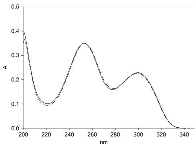
**Figure 2.** UV–vis spectra for one solution containing ligand alone,  $\text{pH}=4.08$  (solid line) ( $[\text{L}]_0=3.39 \times 10^{-4}$  m), and another containing ligand with metal ion,  $\text{pH}=4.13$  (dash-dotted line) ( $[\text{L}]_0=3.39 \times 10^{-4}$  m,  $[\text{Al}^{3+}]_0=9.86 \times 10^{-5}$  m).
